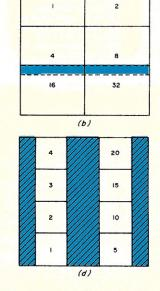
Fig. 1. Practical subdivisions of the Sorcerer character matrix for graphics purposes: (a) For independent point-plotting. Screen resolution  $128 \times 90$ . (b) For creating "filled" areas. Black/white fills unequal. (c) For creating "filled" areas. Fill ratio nearly equal. (d) For vertically single-valued point plots. Screen resolution  $128 \times 120$ .
